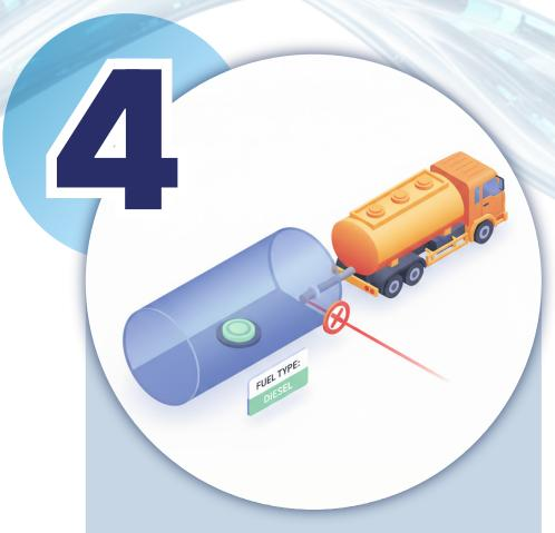
**Optional Fuel Discriminator** prevents mixing in delivery tanks by detecting fuel type in real time.
